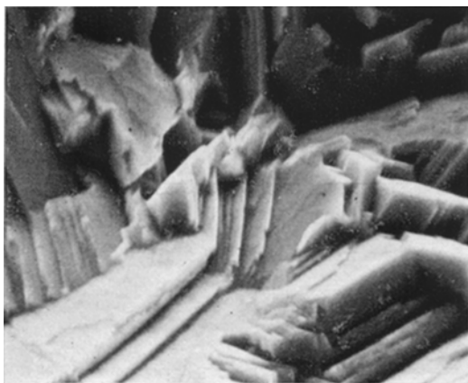
Figure 7 SEM of stage I fracture surface, \times 2100 .
