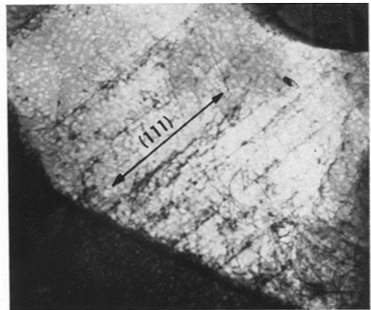
Figure 15 Slip band formation in a necklace grain, \times 15\,500 .
